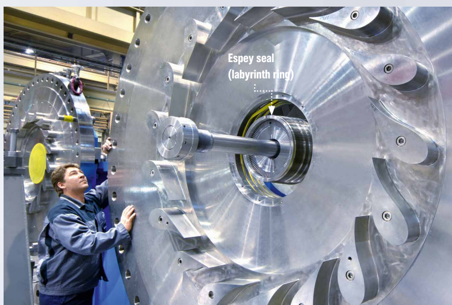
During installation: labyrinth ring shrunk on shaft
