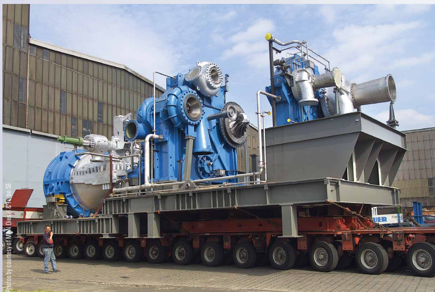
Turbo machinery train for terephthalic acid production: steam turbine, air compressor, integrally geared expander
