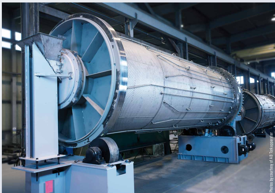
Revolving cylindrical cooler for mining copper (separation copper ore)
