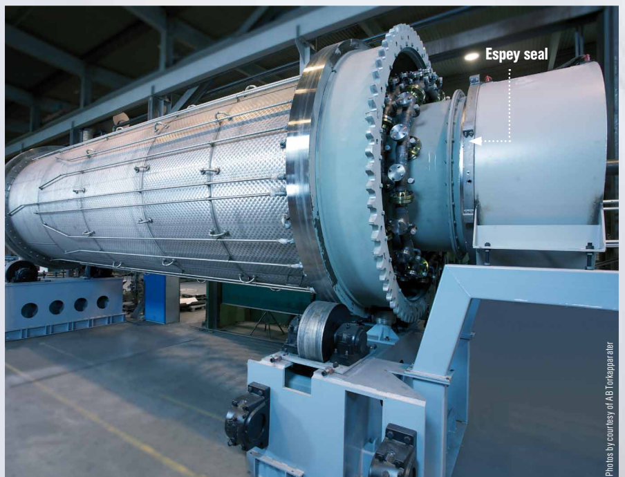
Revolving cylindrical cooler for mining copper (separation copper ore)
